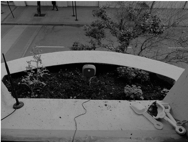
FIGURE 11.2 The Smart Citizen Kit (centre) installed in a resident’s window box.
