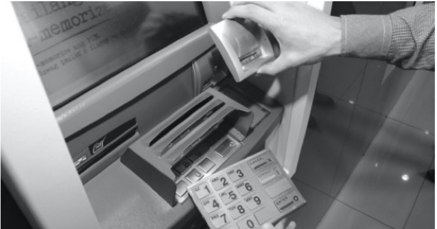
Realistic-looking skimmer overlays for ATMs are sold online.
