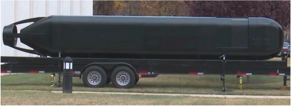
3D-printed submarine hull by the US Navy. (Source: US Department of Energy).
