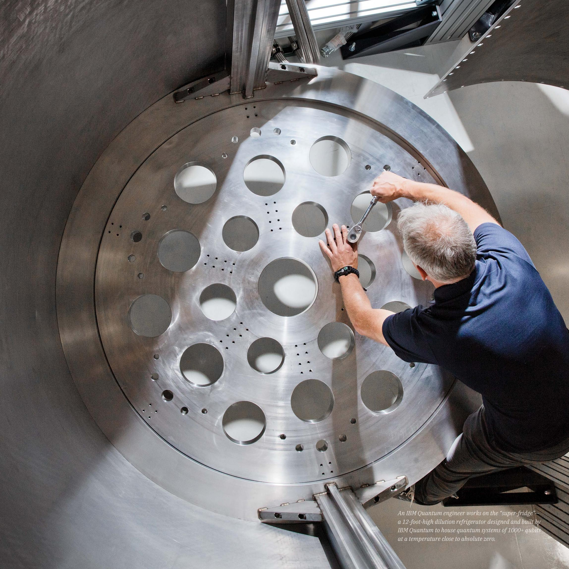
*An IBM Quantum engineer works on the “super-fridge” – a 12-foot-high dilution refrigerator designed and built by IBM Quantum to house quantum systems of 1000+ qubits at a temperature close to absolute zero.*
