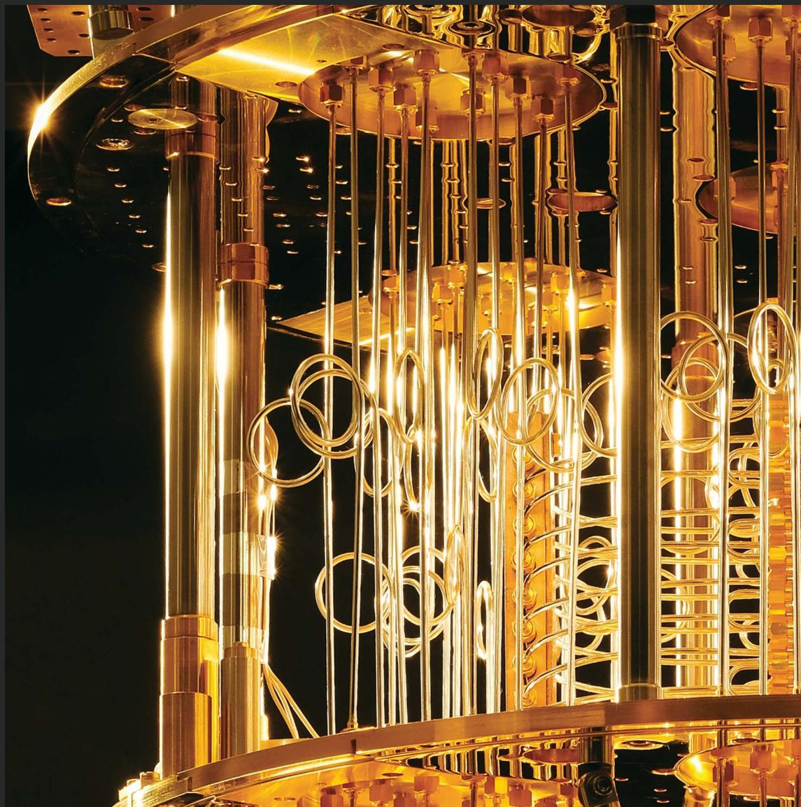
*The internal quantum computing components are held at temperatures close to absolute zero. The microwave control lines contain loops to allow for contraction as the device cools down.*
